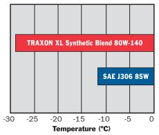
TRAXON XL Synthetic Blend 80W-140 protects equipment better in colder temperatures than 85W grades.
