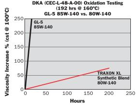
In the DKA oxidation test, product performance is measured by how much harmful viscosity increase will occur over time (therefore, the flatter the line the better). TRAXON XL Synthetic Blend clearly outperforms the GL-5 85W-140 gear oil.
